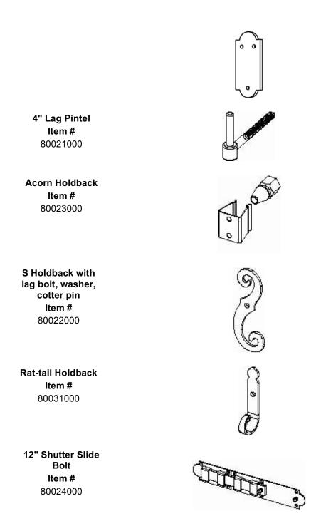
First step is to determine the position of the Pintel on the Window casement. Measure the depth of the surface that the Pintel will be mounted on and the adjacent wall surface. This will determine the Pintel height and Hinge combination that best fits the application.
