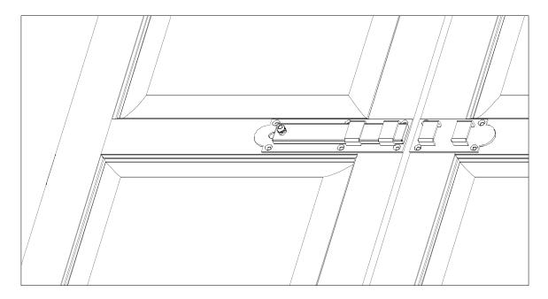
Hang the shutters on the Pintel, check for uniform gap clearance and make sure the shutters are plum.
