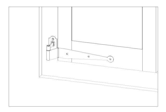
With the shutters in the closed position, locate the Acorn Hold Back Clip 1" down from the upper corner and 11/16' from the edge of the style. Mark the hole location and Drill 1/8" diameter pilot holes through the face of the stiles. Be careful not to drill through the opposite side of the stile. Screw the Hold Back Clip in position.
