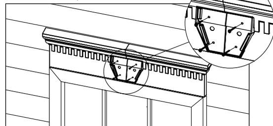
**Note:** shutter fasteners may be used to secure the Keystone Base to the Window Header. If shutter fasteners are being used, drill  $\frac{1}{4}$ " holes through the Window Header and Base as shown below to accept the shutter fasteners.
