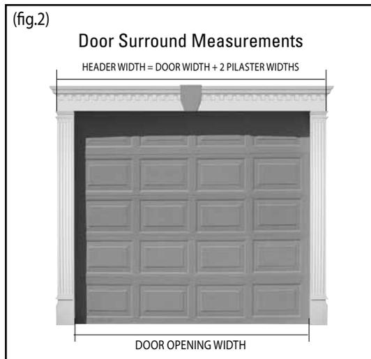
When measuring the width of your door be sure to include the frame.
