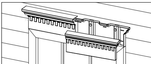
**Note:** If you are installing a classic dentil profile header, and the dentil teeth land on the sides of the keystone, it will need to be trimmed to properly snap in place. If not, proceed to step 7. If yes, trim thinned areas on the Keystone cover as shown below.
